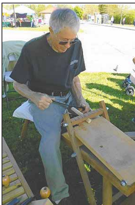
Volunteer George Tyler sits astride a shaving horse while using a drawing knife to make pins for architectural joints.
