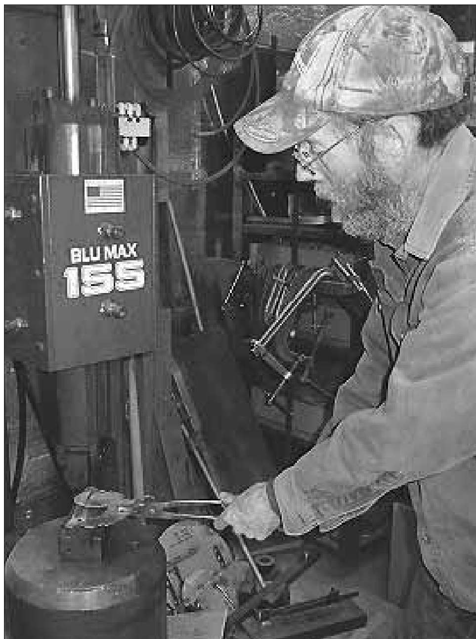
A power hammer gives a piece a distressed look as well as eases the physical work normally done by hammer on anvil.
