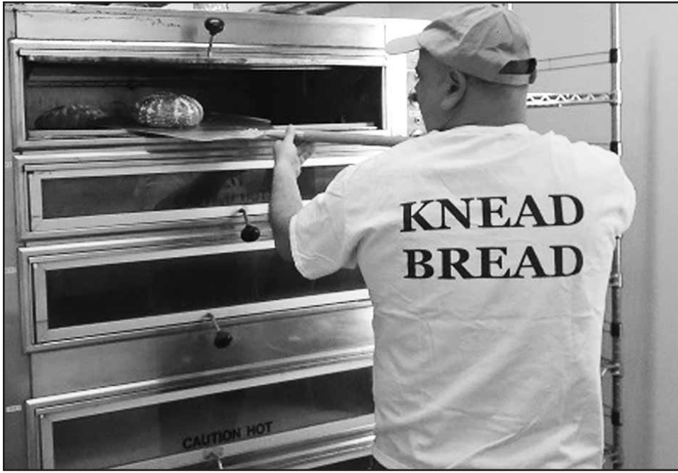
Six ovens with stone bases can cook as many as 50 loaves at a time. The stone ensures evenly-baked crusty bread.
