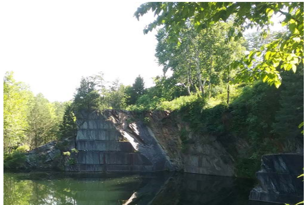
The quarry face reveals a vein of clay wedged into the more prevalent soapstone. Photo by Patrick Healy.
